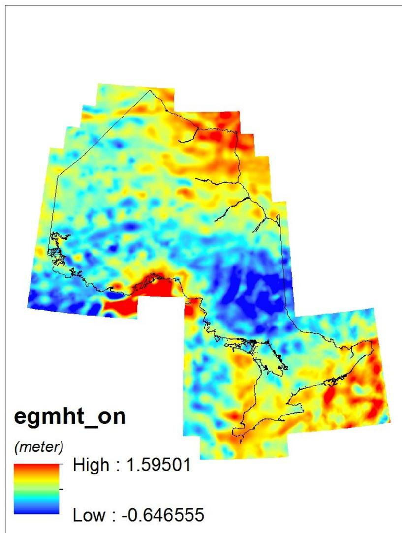
Figure 4: Elevation Distortion between CGVD28 and EGM96
