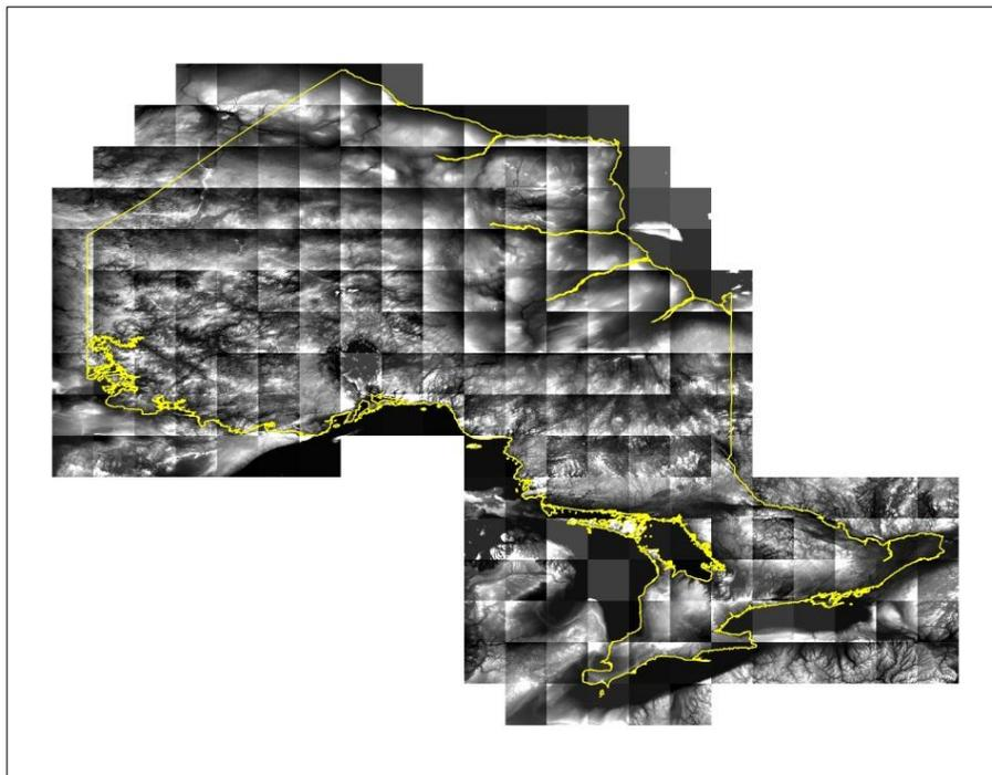
Figure 2: SRTM Tiles Used to Create the Ontario Radar DSM
